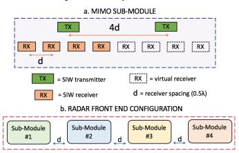
Fig. 1. Representation of the radar: a. sub-module b. complete radar.
