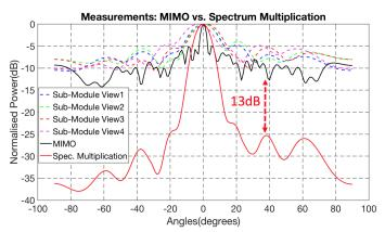
Fig. 4. Measurements for a target at broadside for MIMO radar (4TX by 8RX elements) and spectral beam pattern multiplication (4 sub-radars with 2TX by 4RX for each).
